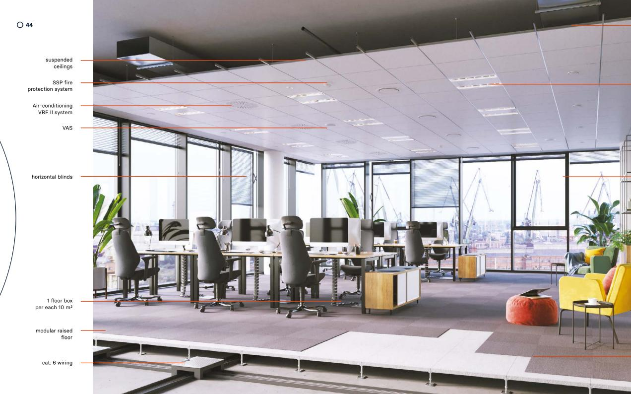
ventilation 40m³/h, with a density of 1 person per 8 m²
